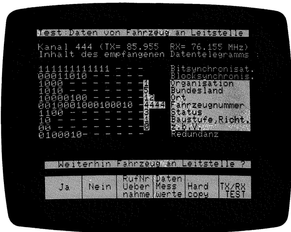
FIG 10 User-specific software controls SCUD for BOS applications.
