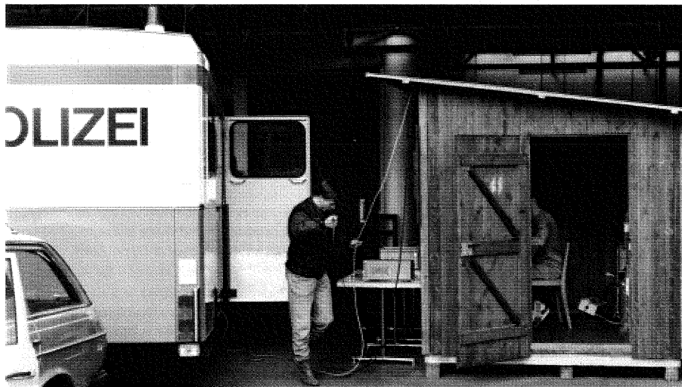
Remote measurement as a special application: the test setup is in the hut, contact to the car telephone is by way of a 10-meter cable and a special interface (devised by the PTT).
